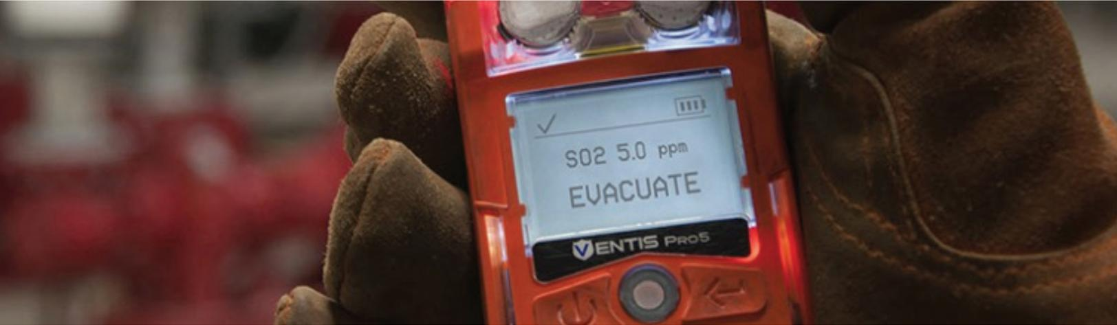
Gas detectors are lifesaving instruments that must be worn in your breathing zone to be effective. OSHA defines the breathing zone as “a hemisphere forward of the shoulders within a radius of approximately six to nine inches,” so a collar, lapel, or outside breast pocket is usually a good option. This location also keeps the instrument visible so you can see alerts if your hearing is impaired while working in a high-noise environment.
